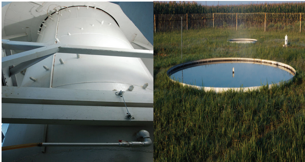
Fig. 9. 6. The weighing lysimeter (left) and the biggest evaporation tank (20M 2 in area) at the evaporation observation site (right) of YCES
